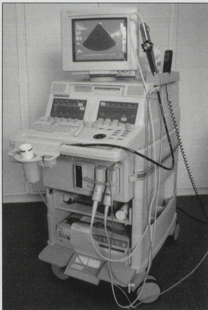
Figure 1. Echocardiographic imaging console with transoesophageal probe. The imaging system is capable of performing two-dimensional and M-mode imaging together with colour flow, continuous wave and pulsed Doppler.
